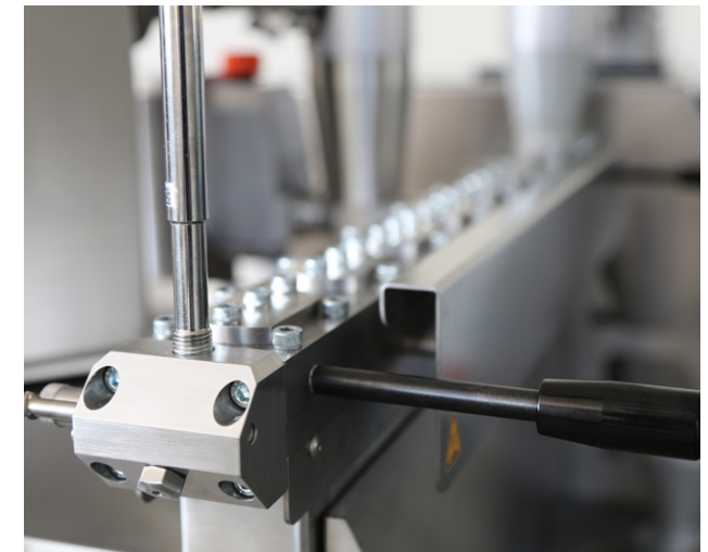
Segmentation of barrel to match process requirements.
