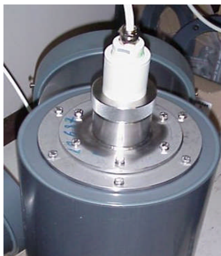
Typical mounting arrangement of the LB6365 in a 300mm diameter ventilation duct.
