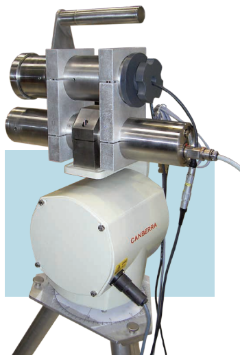
Figure 3 CARTOGAM coupled with a CZT detector.
