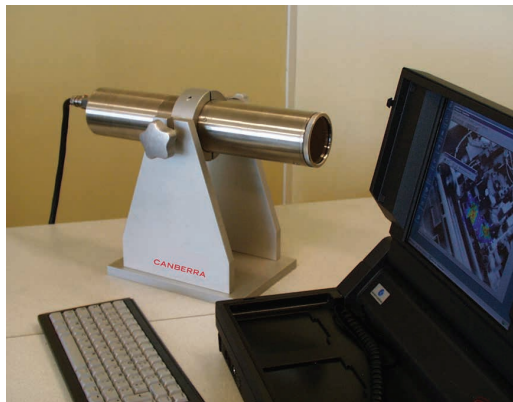
Figure 2 CARTOGAM measurement head with its PC and scheme of the image processing.
