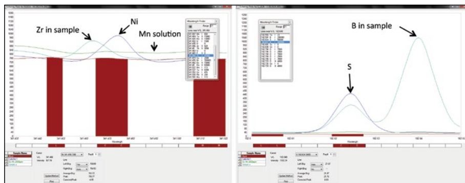
Figure 1. Ni 341.476 nm and S 182.624 nm sub-arrays obtained for the sample and 2000 mg/L Mn solution
