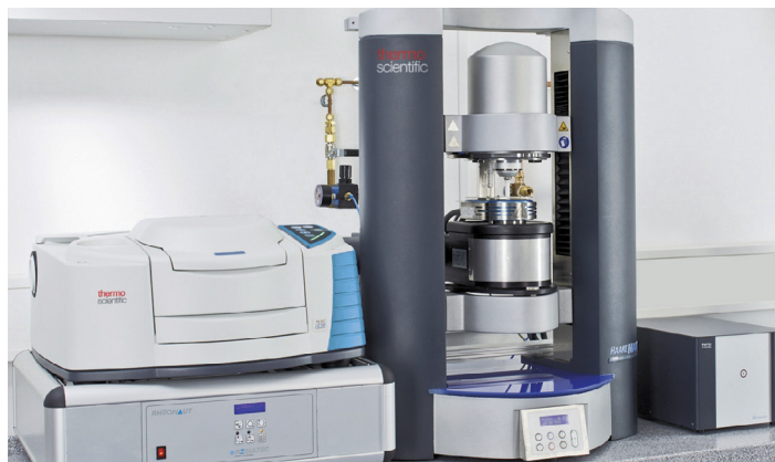
Figure 1: Setup with the HAAKE MARS Rheometer, Rheonaut module* and Thermo Scientific Nicolet iS20 FTIR spectrometer
