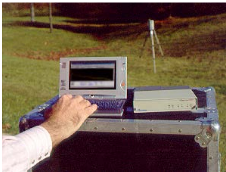
Figure 2 The InSpector 2000 MCA with its Laptop Control and Analysis Computer and Germanium Detector in a Big MAC Cryostat.
