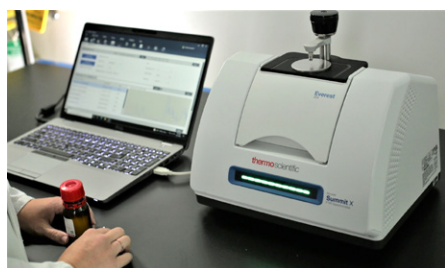
Figure 1. Nicolet Summit X FTIR Spectrometer with Everest Diamond ATR Accessory, powered by OMNIC Paradigm Software.
