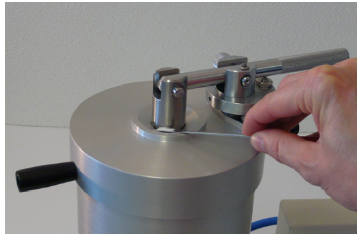
Introducing the powder in the Nebula for a proper dry dispersion
