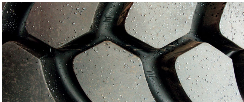
Figure 1: Carbon black rubbers, such as this tire, represent a challenging sample for infrared analysis
