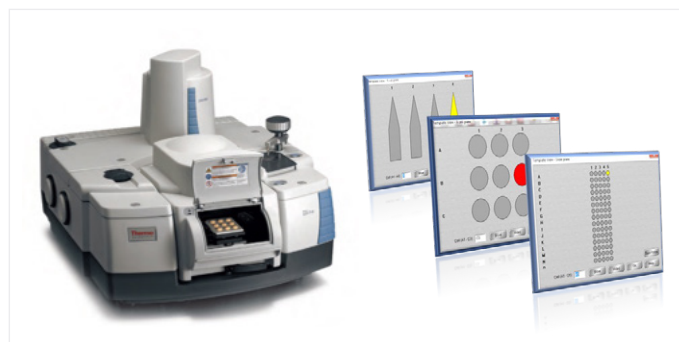
Figure 1. Nicolet iS50 FTIR Spectrometer with the iS50 Raman Accessory (left). Available analysis templates (right).
