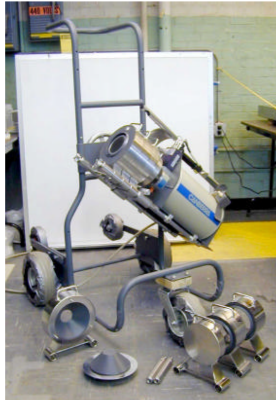
Figure 2-2. ISOCS cart with detector, cryostat and modular shield system
