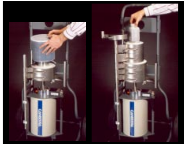
Figure 3. ISOCS used to assay Marinelli beakers and small sample containers
