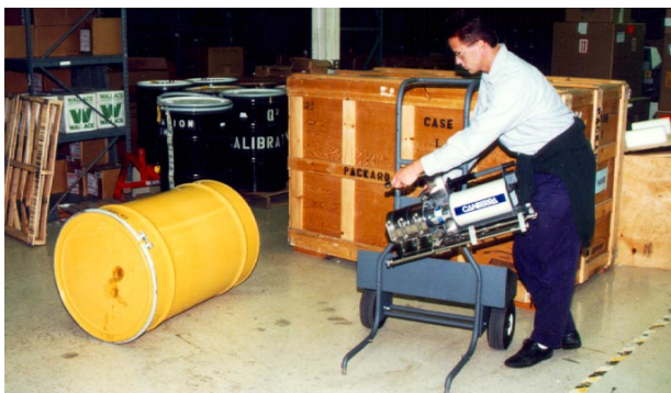
Figure 1. ISOCS used to quantify radioactivity in a 200 liter drum
