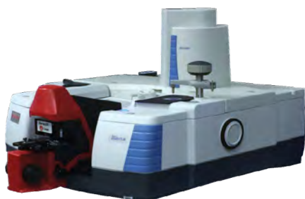
Figure 1: Nicolet iS50 FTIR spectrometer with the SurveyIR microspectroscopy accessory in the sample compartment.
