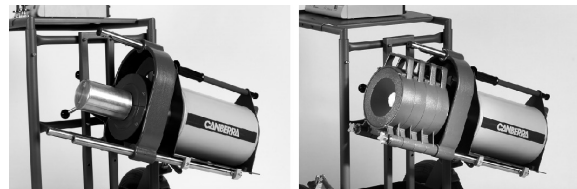
5a: The detector and mounting assembly. Note that the detector has the RDC chamber and that the backshield is installed.
