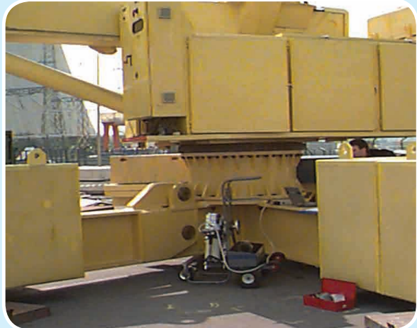
Using the ISOCS system to characterize a crane in nuclear plant in US, demonstrating the capability to characterize massive objects.
