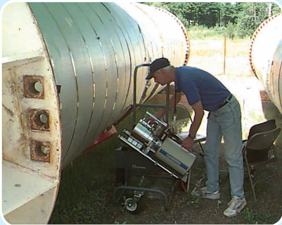
Characterization of heat exchangers for free release at Seabrook NPP (USA).
