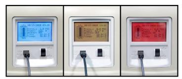
Blue LCD backlight: Unit operates normally, no action is required.
