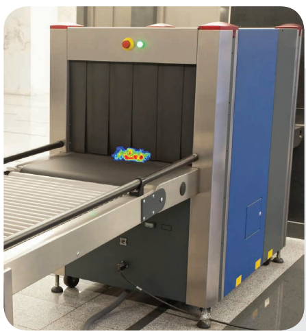
Curtain X-Ray leak check.
