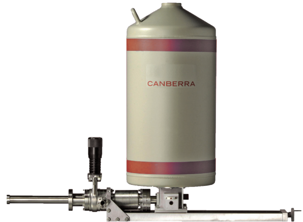
100 mm 2 Ultra-LEGe detector in windowless retractable cryostat
