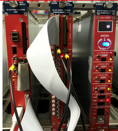
Fig. 2: Picture of the used CAEN boards, from left to right, N6741 Peak Sensing ADC, N1168 Fast Shaping Amplifier, and N1470 power supply unit.
