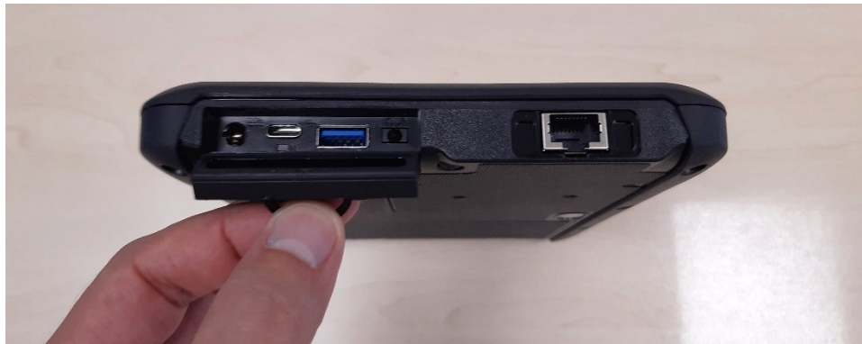
Figure 5.1: Side USB port of the control tablet
