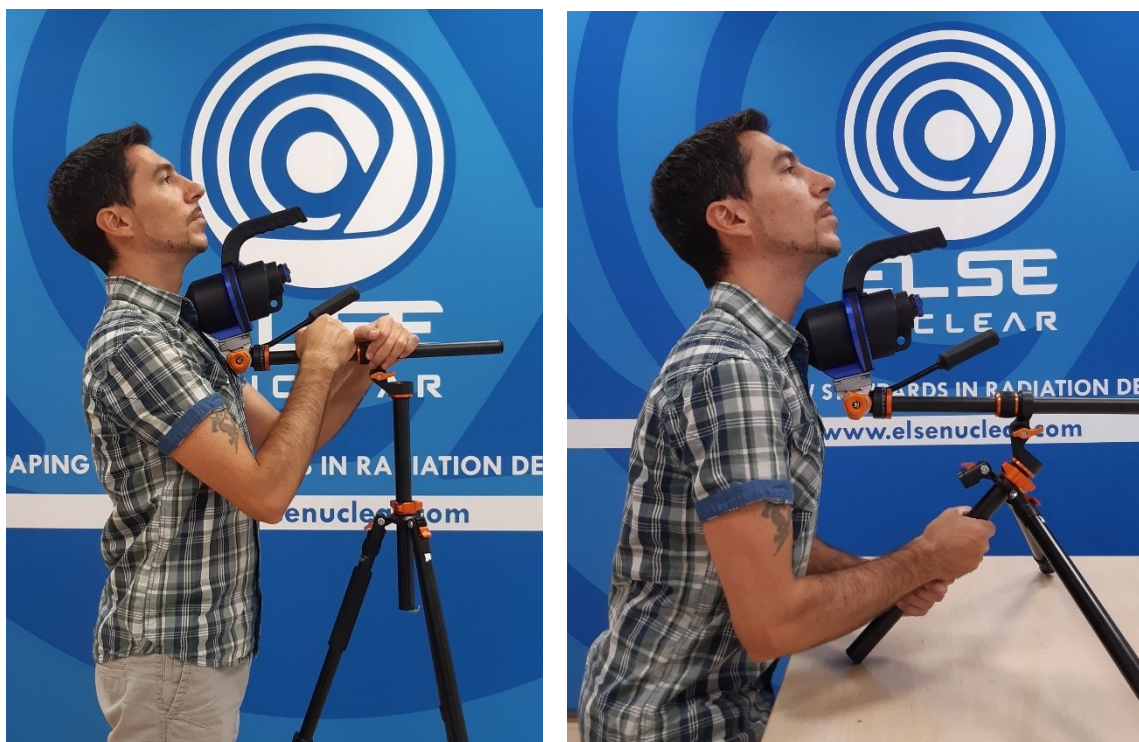
Figure 3.1: Examples of measurement position for standing and table-top configurations
