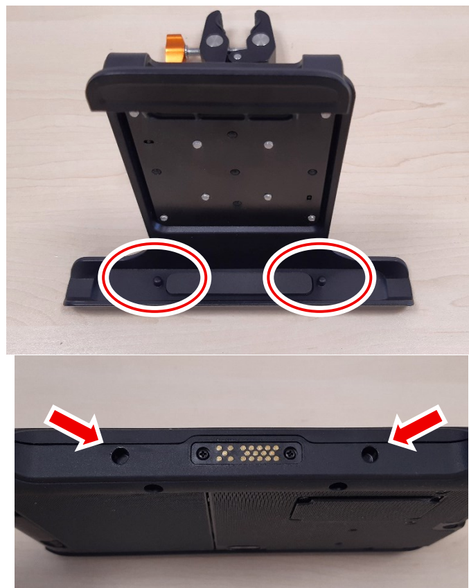
Figure 3.4: Cradle holding pegs and tablet mounting holes
