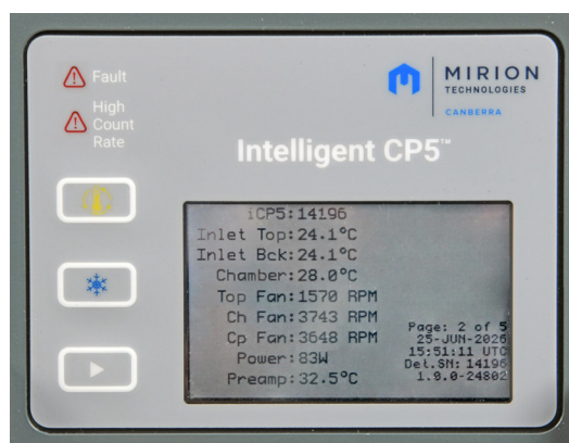
Figure 1: iCP5 top panel: picture of the keypad and LCD display
